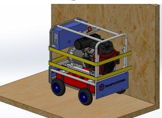
NOTE: Example of strapping in an enclosed trailer.
