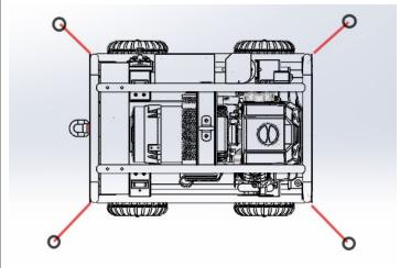
Be sure machine is fully secure utilizing straps that are properly specified for the machine's weight.
