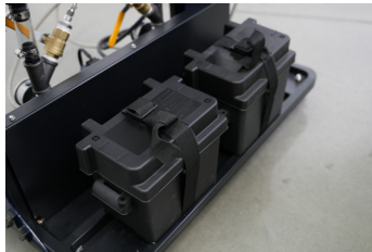
DUAL ON-BOARD 24V BATTERIES
