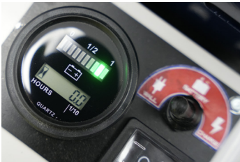
BATTERY LIFE INDICATOR AND EASY FLIP ELECTRICAL SYSTEM
