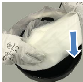
3- Insert the new Infinity Bag with the inner part facing upwards.
