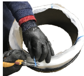
4- Cut and remove the Infinity Bag closing bands.
