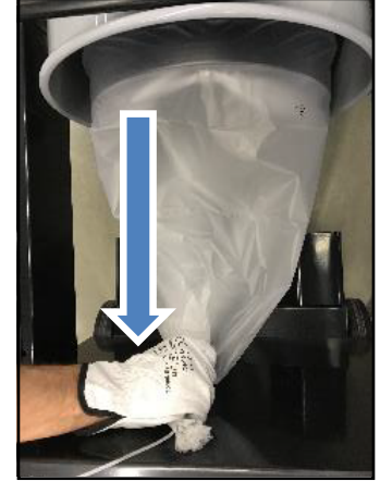
3 - Pull the Infinity Bag end to make a new bag.
