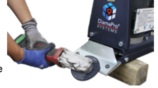
FIG 3-M Sharpening with a fine-toothed file
